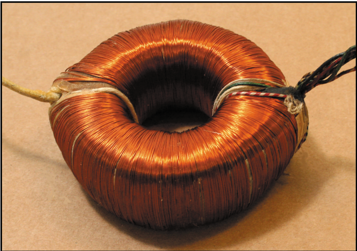
Fig. 10 Here are a couple of photos of the coil directly after the wrapping was removed. The outer winding has no other wrapping or shield.
