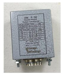
**Vintage Windings VW-P-50:** Bifilar 1:5 Ratio Transformer with larger core than an HS-50. Can handle dc on secondary. Better than 90db shielding. With CT.
