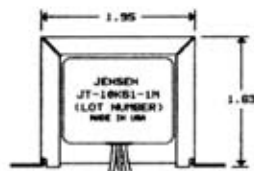
#26 AWG (17-34) UL STYLE 1061 COLOR CODED WIRE LEADS. 8" MINIMUM LENGTH
