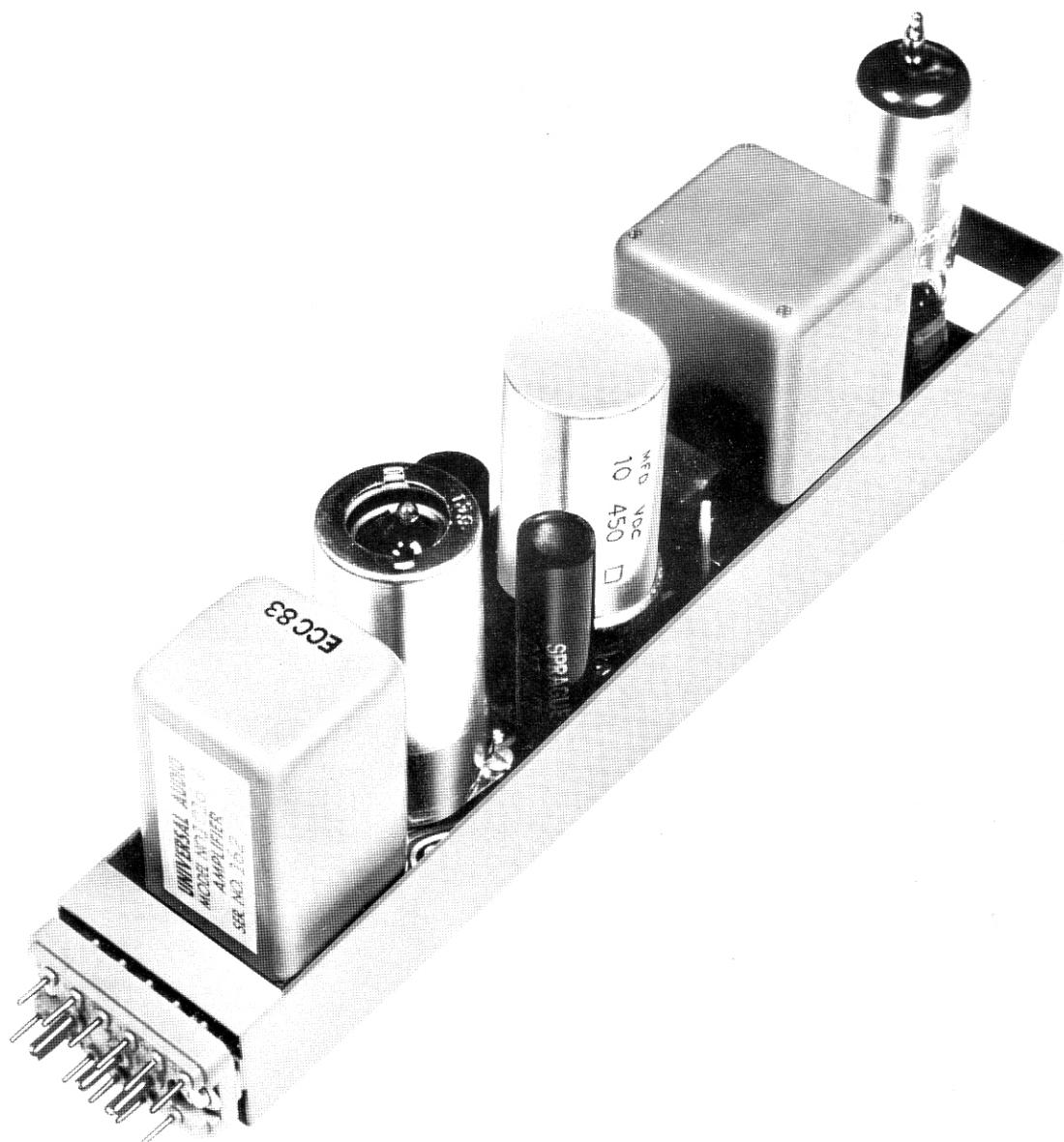
The 1016 is a miniature (1 1/2" wide including tray), plug-in amplifier. One unique feature of this unit is that, unlike the normal amplifier, this item is suitable for all applications; as a microphone preamplifier, a booster amplifier, or a line level program amplifier in any professional audio system. This allows for standardization and improved utility.
