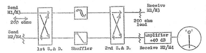
M1 - M2 Send unbalanced to M1. Receive from M2 as shown.
