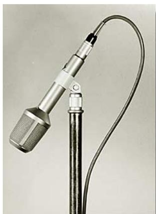
In an even (diffuse) sound field, no appreciable change in on-axis (0 degrees) response occurs when switching from omni to cardioid pattern. Also, when the backside capsule is added (for omni), there is less than a 10% increase in output voltage from the microphone.
