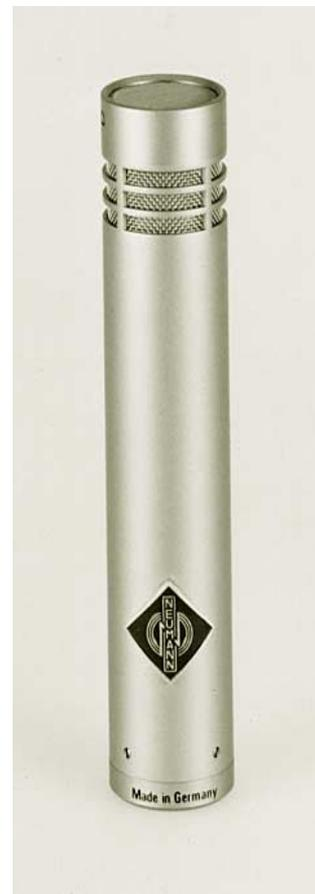
The KM 84 was designed with a 10 dB attenuation switch, therefore allowing the microphone to be used up close with loud instruments. By placing the pad at the gate of the field-effect transistor (FET), this "pre-attenuation" prevents the hot capsule signal from overloading the front end of the amplifier. With the switch on, a sound pressure level of 130 dB can pass through without distortion.
