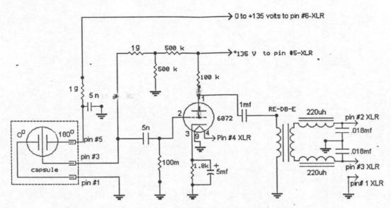
Schematic Diagram of L-47MP Gold Tube Microphone
