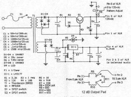
Schematic Diagram of L-47MP Power Supply
