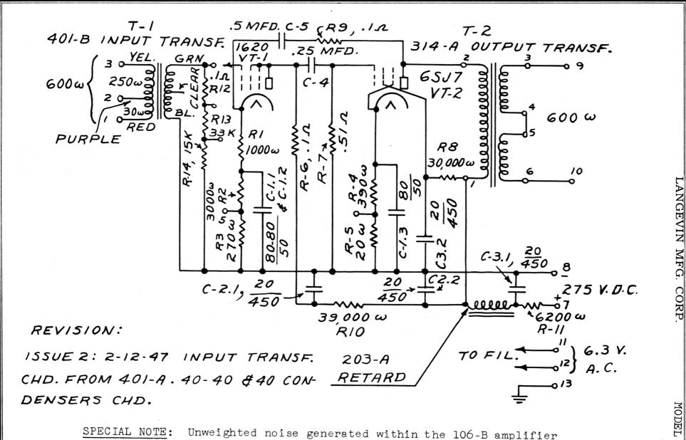
is equivalent to an input signal of -118 dbm (db
