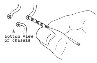
Use a small metal twist drill (1/8" dia. or less) to clear the hole only in the fillet of solder.
