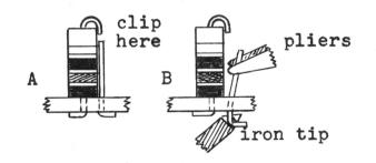
place iron on fillet and push wire through the hole until the hook can be clipped off.
