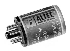
The 1579A Preamplifier is designed for use with magnetic phono pickups and will equalize them to meet the RIAA standard. Sensitivity is 5 millivolts for 70 millivolt output at 1 kHz. Output is +8 dBm at less than 0.5% THD. Input impedance is 47,000 Ohms and the power required is 12V dc at 11 mA. The 1579A plugs into a standard octal socket and has a diameter of 1 5/16" and a seated height of 1 13/16".
